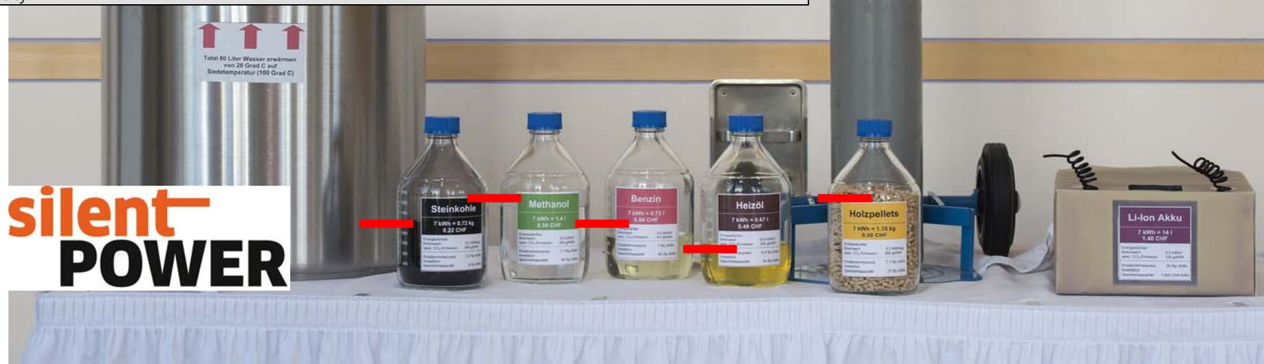
**Comparison of storage media/energy sources: On the left: cooking pot with 80 litres of water to be heated from 20 to 100 °C boiling point. The energy required: 7 kWh. This amount is contained in each of the lined up energy sources or energy storage media. Red markings on the left side of the 2-litre bottles show the corresponding fill level.**
